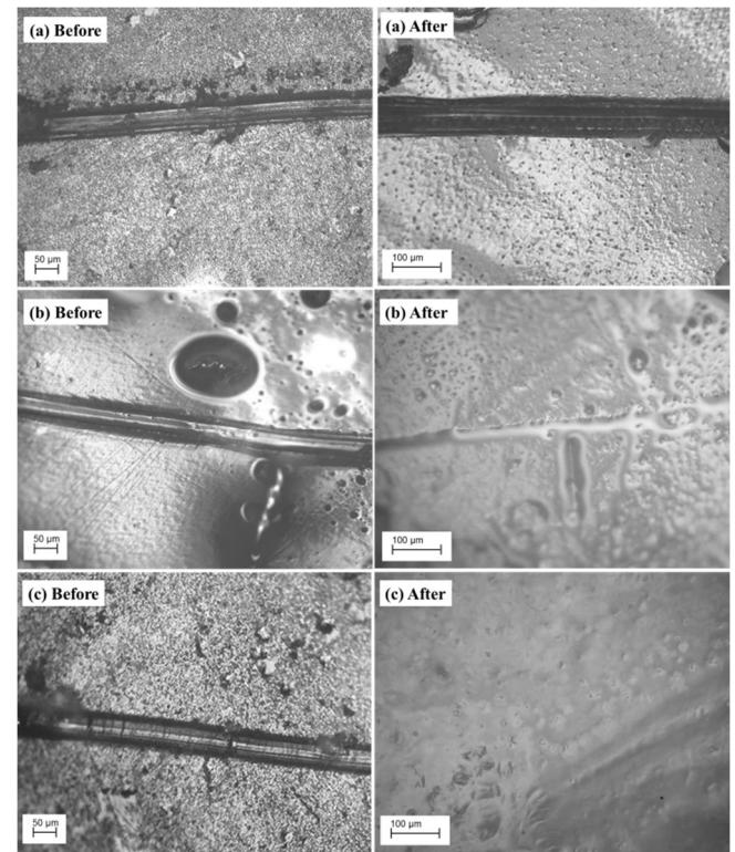
Fig. 2: Micrographs of self-healing behavior of PCLU coatings before and after thermal stimulating at 90°C , (a) PCLU10, (b) PCLU50, and (c) PCLU90.
