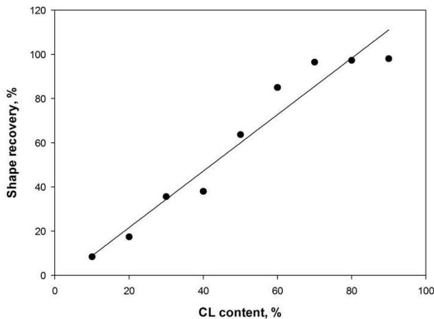
Fig. 1: Effect of CL content on shape recovery of PCLU coating
