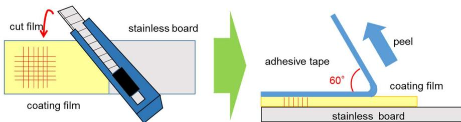
Figure 4. Image of cross-cut test.
