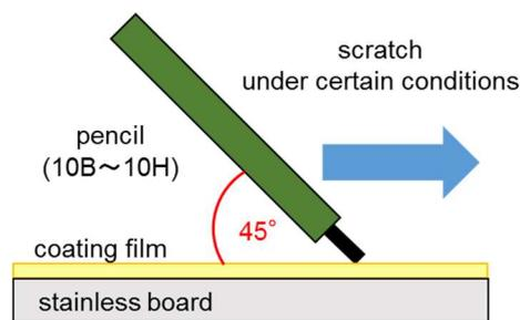
Figure 3. Image of pencil hardness test.
