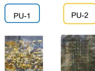
Figure 6. Results of cross-cut test [PU-1 (left) and PU-2 (right)].
